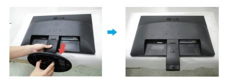
**5.** Pushing the PUSH button, Take the stand body from hinge body.
