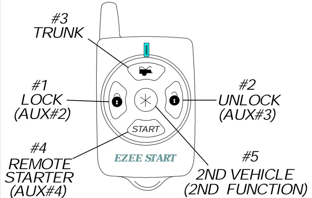
The transmitter supplied with the EZ-45DP II/55DP II system has five buttons. The button configuration of the EZ-45DP/55DP II is Factory-set and unchangeable. See Page 12 for additional information on how to use your remote to operate a second vehicle equipped with a EZEE START system.
