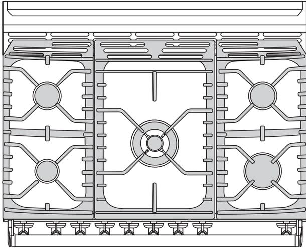
Each grate is different. Make sure that the grates are in the correct position and sitting down.
