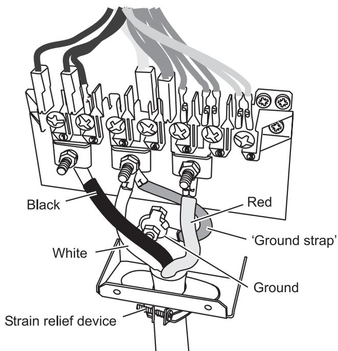
The neutral or ground wire of the power cord must be connected to the neutral terminal located in the center of the connector block. The power leads must be connected to the outside terminals.
