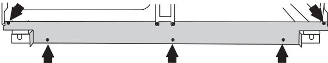
Fit the outer plinth (2 screws 1 each end) to the inner plinth. The height of the outer plinth can be adjusted by sliding it up or down via the slotted hole.
