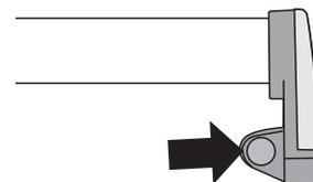
Fix the front handrail in position. Fit the plastic blanking plugs to the fixing holes.
