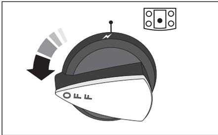
Keep holding the knob pressed in to let the gas through to the burner for few seconds. The igniter should spark and light the gas.
