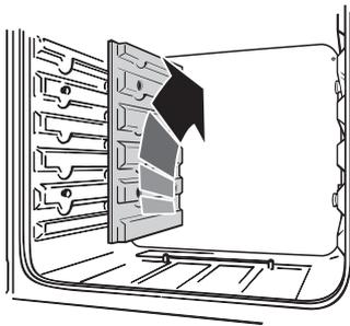
Once the linings are removed, the oven enamel interior can be cleaned.
