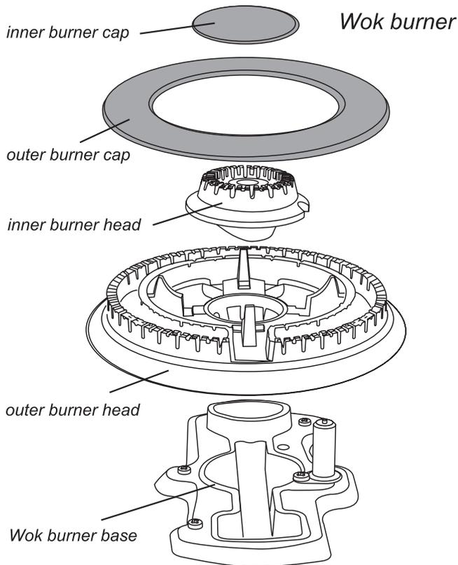
When reassembling a Wok burner, turn over the large base ring and find the 'D' shaped area.
