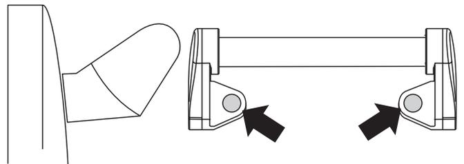
Fit the plastic blanking plugs to the fixing holes.
