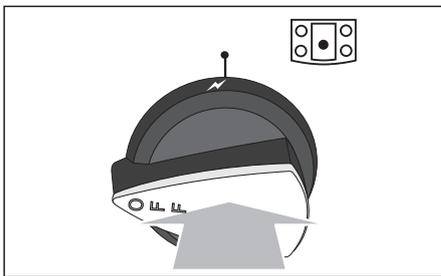
If, when you let go of the control knob, the burner goes out, the safety device has not held in. Turn the control to the off position and wait one minute, then try again this time holding in the control knob for slightly longer.
