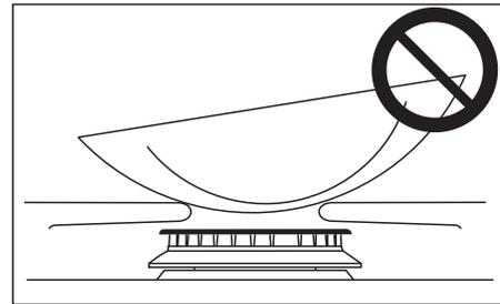
Avoid using unstable and misshapen pans that may tilt easily and pans with a very small base diameter e.g. milk pans, single egg poachers. The minimum pan diameter recommended is 4<sup>3</sup>/<sub>4</sub>".
