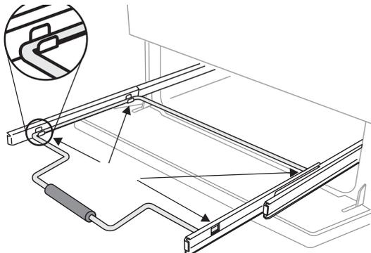
For each side, support the side rail with one hand and with the other hand lift the frame up and out of the side clips.
