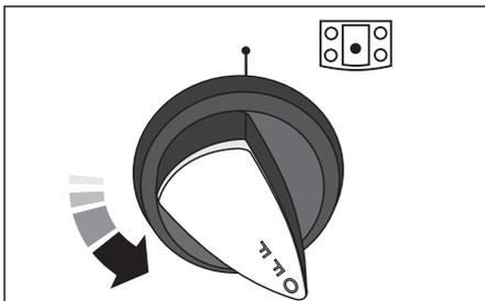
Adjust the flame height to suit by turning the knob. On this range the low position is beyond high, **not** between high and off. The 'LO' marks the low position. Turn the knob towards it after the contents of a pan have boiled.
