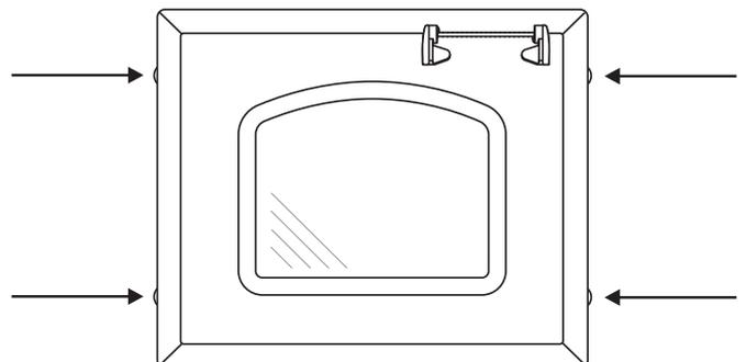
The fixing screws have a recessed hexagon socket in the head. A hexagon key to fit the screw is supplied in the instruction pack.
