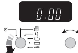
To set the clock to read the time of day turn and hold the Setting knob to the clock symbol (⌚) and at the same time turn the Adjusting knob left or right until the clock shows the time of day. This is a 12 hour clock. Let go of the Setting knob and it will spring back to the vertical (⏻) oven manual setting.
