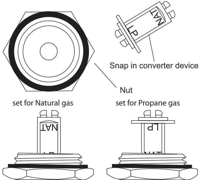
The snap in converter device is marked to show which gas it is set for. Make sure the device is secure in the base of the nut and refit the nut to the regulator.
