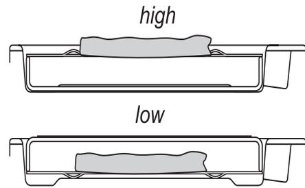
For best results preheat for 2 minutes with the broiler pan in position. After placing your food on the broiler pan grid, slide the broiler carriage. Adjust the heat to suit by turning the knob.
