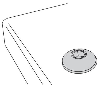
Remove the two fixing screws (3mm hexagonal socket head) and nuts that pass through the top of the rear flue grille.
