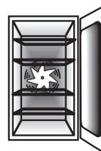
The fan in the right hand Tall oven circulates hot air continuously, which means faster more even cooking. The recommended cooking temperatures for a fanned oven are generally lower than a non-fanned oven.
