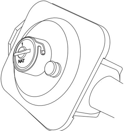
The regulator has a bayonet mounted top cap. Using a small coin press in and turn the cap to remove it.
