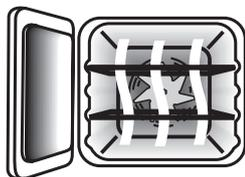
The left hand oven is a Multi-function oven. As well as the oven fan and fan element, it is fitted with two extra heating elements, one visible in the top of the oven and the second under the oven base. Take care to avoid touching the top element and element deflector when placing or removing items from the oven. For more detail on this oven see the section 'Multi-function oven'.
