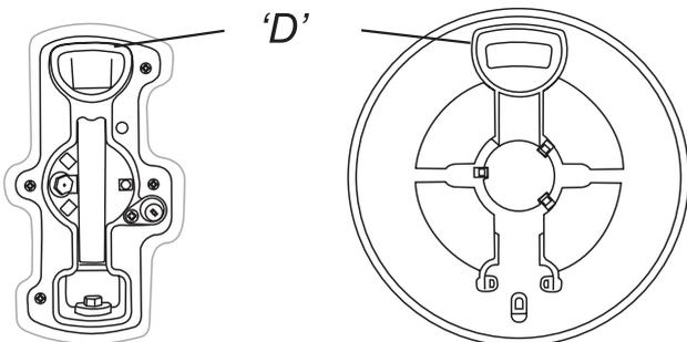
Turn the head until the 'D' matches the one on the burner base. Turn the head over and place it on the burner base.
