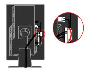
7. Wrap the Cable Wrapper around the cables.
