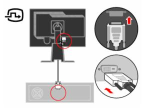
3. Connect the analog signal cable to the D-SUB connector of the monitor and the other end on the back of the computer.
