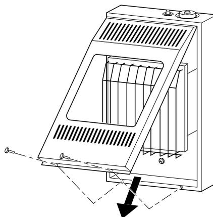
**Figure 10 - Removing Front Panel Of Heater**
