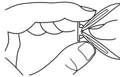
**Figure 6 - Folding Anchor**
