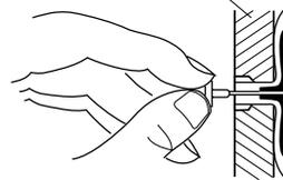
**Figure 7 - Popping Open Anchor Wings For Thin Walls**
