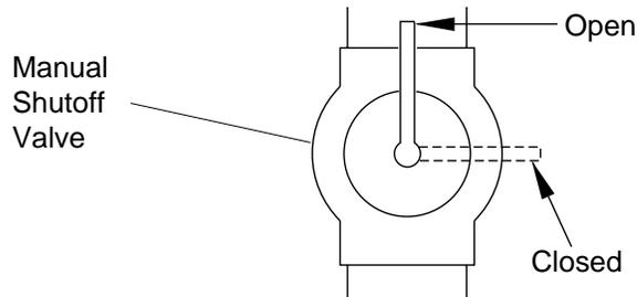
**Figure 13 - Manual Shutoff Valve**
