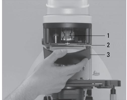
**Fig. 26** Inserting the filter or reflector cubes
