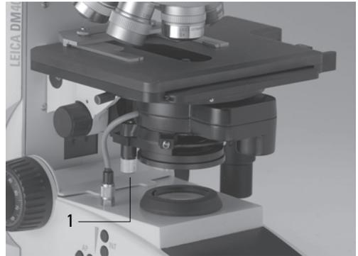
**Fig. 28** Inserting the compensators
