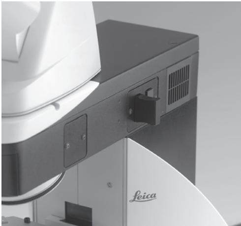
**Fig. 76** Inserting the excitation manager
