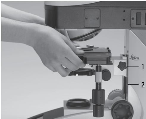
**Fig. 4a** Pol rotating stage\* and Pol 3 attachable mechanical stage\*
