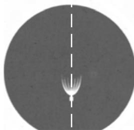
**Fig. 55** Direct arc image and mirror image in target position (in reality, the image is less focused)
