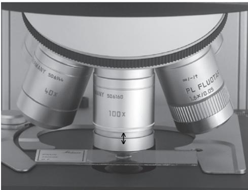
**Fig. 63b** Immersion objective, locked
