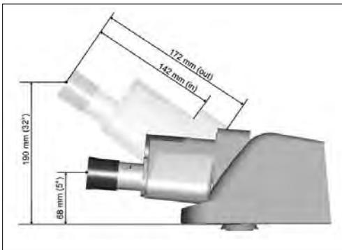
**Fig. 62** BDT25+ tube with digital camera
