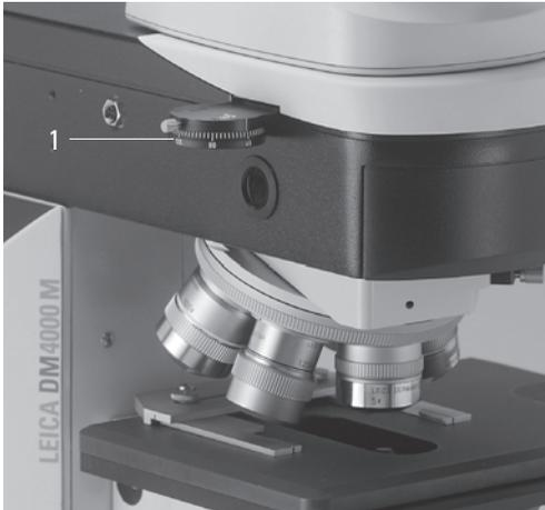
**Fig. 31** Inserting the objective prism slide
