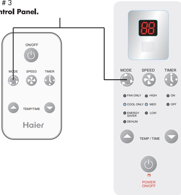
Once the mode function is established, you will have to set the fan speed. (See fig. #4) Every time you press the SPEED button, fan speed will change between LOW, MED, and HIGH.
