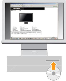
6. To optimize your monitor image, press the Automatic Image Setup key. **Automatic image setup** requires that the monitor is warmed up for at least 15 minutes. This is not required for normal operation.
