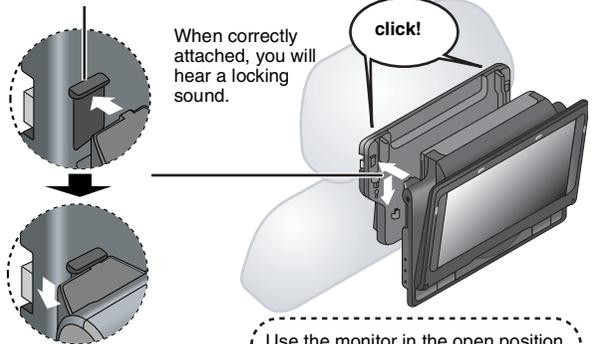
Diagram of the attached bracket and unit
