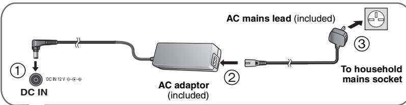
The unit is in the standby condition (the [⏻] indicator lights) when the AC mains lead is connected. The primary circuit is always "live" as long as the AC adaptor is connected to an electrical outlet.
