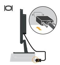
3. Insert the power cord into the monitor, then plug the monitor power cord and the computer cord into grounded electrical outlets.
