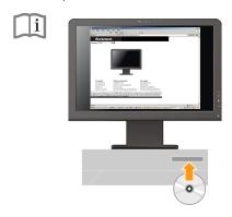
6. To optimize your monitor image, press the Automatic Image Setup key. **Automatic image setup** requires that the monitor is warmed up for at least 15 minutes. This is not required for normal operation.
