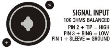
The Neutrik® Combo connector accommodates ¼” phone plugs, XLR, TRS. Please note that PIN 2 is hot! If you are using an unbalanced connection make sure and wire PIN 1 and PIN 3 together at the source end.
