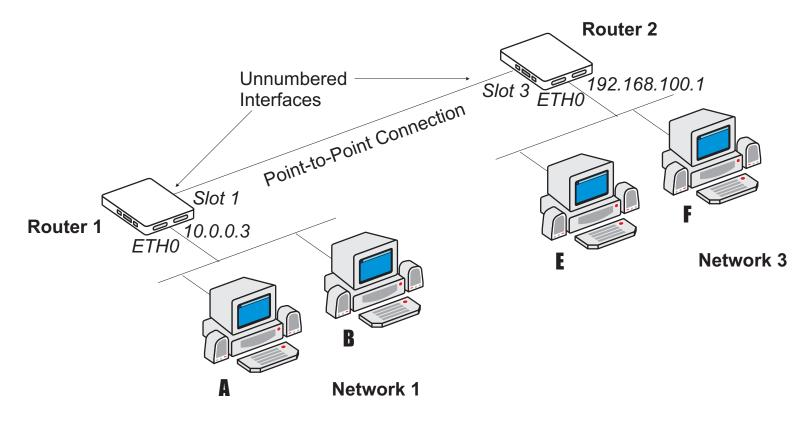
FIGURE 9.2 STATIC ROUTING EXAMPLE 2
