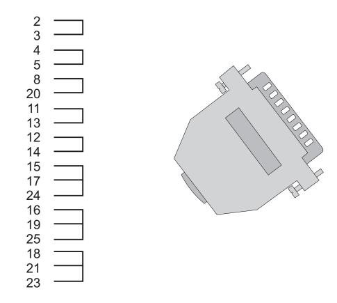
FIGURE B.8 LOOP-BACK CONNECTOR - DB-25 MALE
