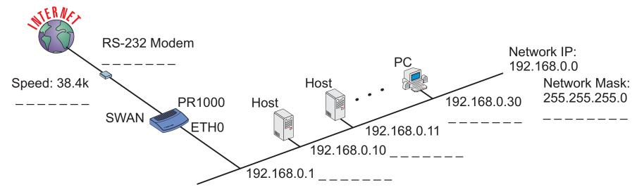
FIGURE 4.1 CONNECTION TO ACCESS PROVIDER USING A SWAN INTERFACE AND A MODEM
