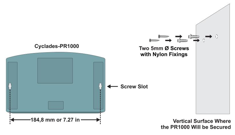
FIGURE 2.5 POSITIONING OF SCREWS
