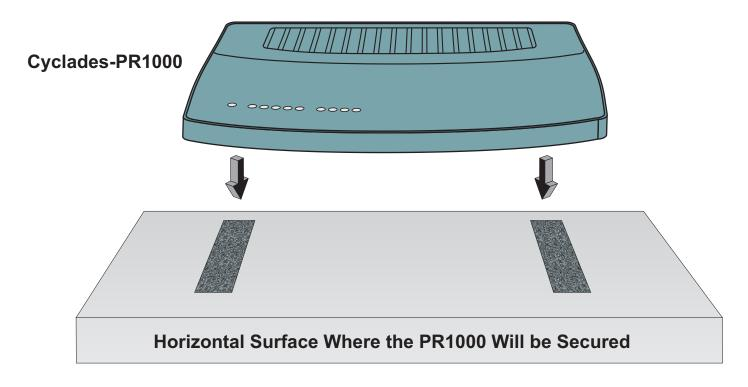
FIGURE 2.4 HOW TO ATTACH THE PR1000 TO A HORIZONTAL SURFACE
