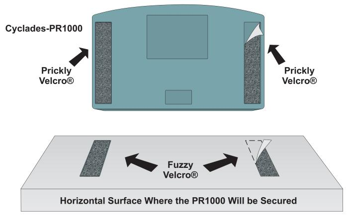
FIGURE 2.3 HOW TO ATTACH THE VELCRO® STRIPS
