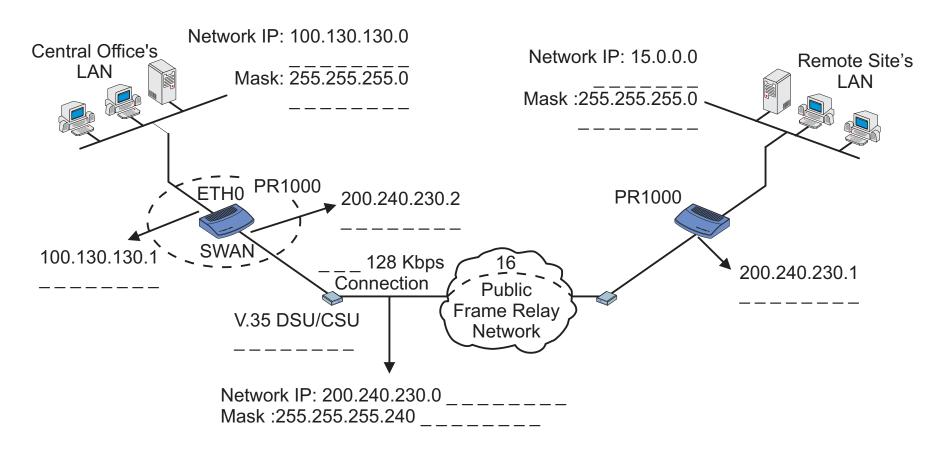
FIGURE 4.11 CENTRAL OFFICE AND REMOTE SITE CONNECTED USING SWAN INTERFACES
