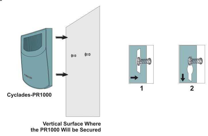
FIGURE 2.6 HOW TO ATTACH THE PR1000 TO A VERTICAL SURFACE
