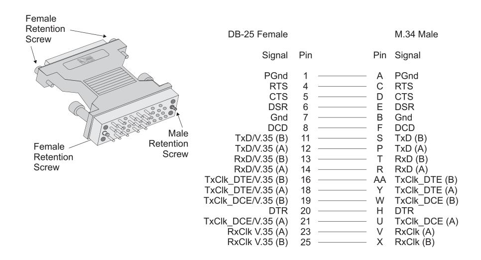
FIGURE B.6 DB-25 TO M.34 ADAPTER - DB-25 FEMALE TO M.34 MALE
