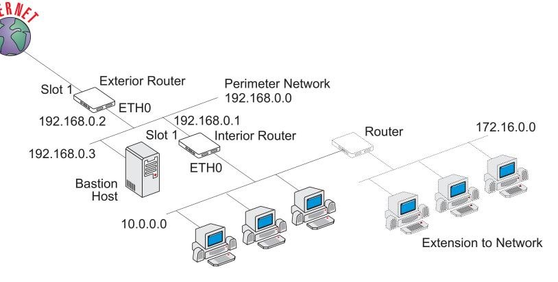
FIGURE 12.2 FIREWALL EXAMPLE
