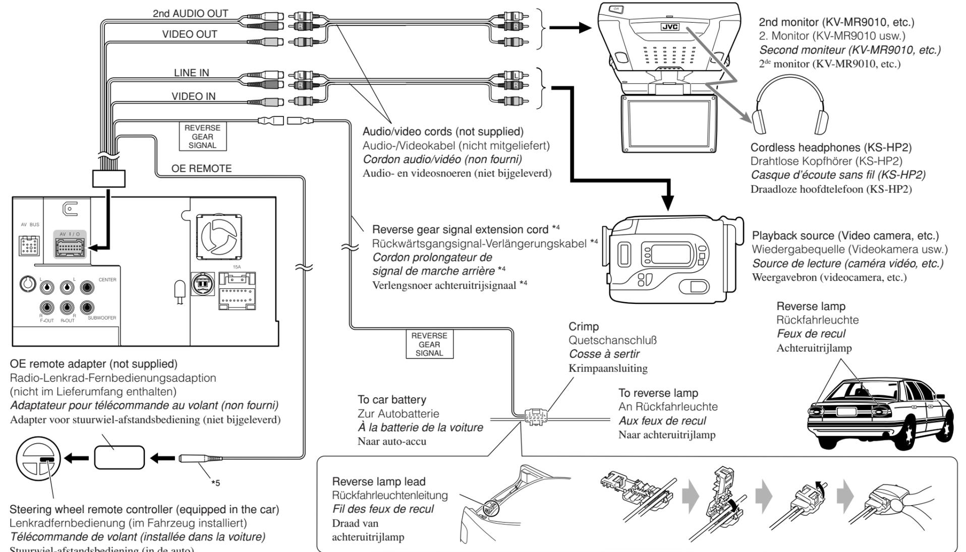
\*4 Required only when connecting a rear view camera to VIDEO IN plug.
