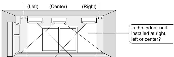
**NOTE:** If the indoor unit is installed more than 19-3/4 inch (50 cm) away from the side walls, cabinets or other nearby objects, set the slide switch to the "center" position.
