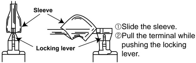
(2) The terminal with this connector has the locking mechanism.
