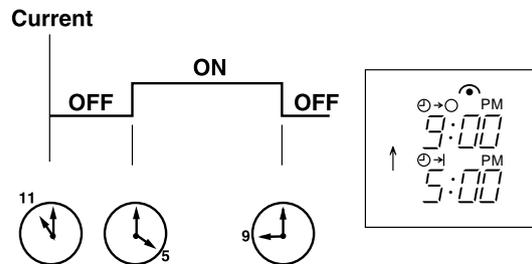
**NOTE :** If the main power is turned OFF or a power failure occurs while ON/OFF timer is active, the timer setting is cancelled. As these models are equipped with an auto restart function, the air conditioner starts operating with timer cancelled when power is restored.
