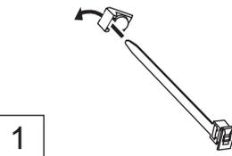
To secure cables connected to Terminals, wrap the cable fixing band around them then pass the pointed end through the locking block, as shown in the figure. **While ensuring there is sufficient slack in cables to minimize stress (especially in the power cord), firmly bind all cables with the supplied fixing band.**
