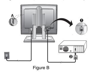
3. Connect the power cord to the monitor and then plug the power cord into a properly grounded outlet. Next, reconnect the power cords to your computer and all attached devices.
