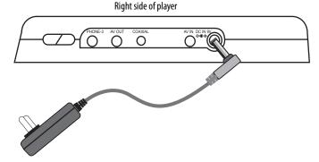
2 Plug the AC adapter plug into a 110 V power outlet.
