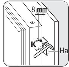
Remove the brackets and mark a distance of 8 mm from the outer edge of the door where the nail must be fitted (K).
