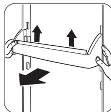
Gradually pull the shelf in the direction of the arrows until it comes free, then reposition as required.
