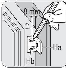
Open the appliance door and the kitchen furniture door at an angle of 90°. Insert the small square (Hb) into guide (Ha). Put together the appliance door and the furniture door and mark the holes.
