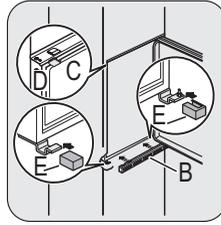
Attach the covers (C, D) to the lugs and the hinge holes. Install the vent grille (B). Attach the hinge covers (E) to the hinge.
