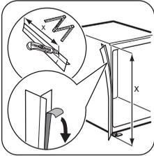
If necessary cut the adhesive sealing strip and then apply it to the appliance as shown in figure.
