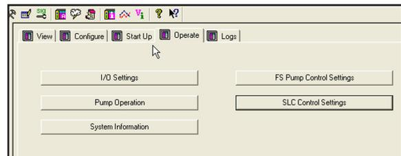
TechView allows easy connection to any ControlWave PLC/RTU through serial or Ethernet ports. The utility is essentially a web page browser that really simplifies menu navigation and PLC/RTU configuration.
