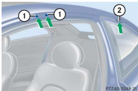
Mount the roof rack only between the fastening points **1** and in the recess of the rubber strip **2**.
