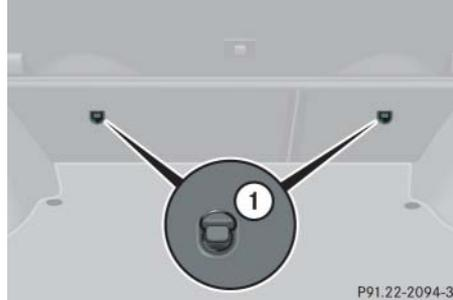
Anchorage rings **1** are located on the back side of the rear backrests and on the floor behind rear seat.
