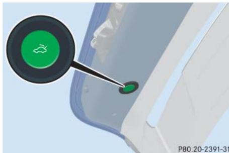
The emergency release button is located in the trunk lid.
