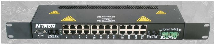
The *N-TRON*<sup>TM</sup> 526FX2 Series Industrial Ethernet Switch offers outstanding performance and ease of use. It is ideally suited for connecting Ethernet enabled industrial and/or security equipment and can be optionally configured with advanced Ethernet communication management functions
