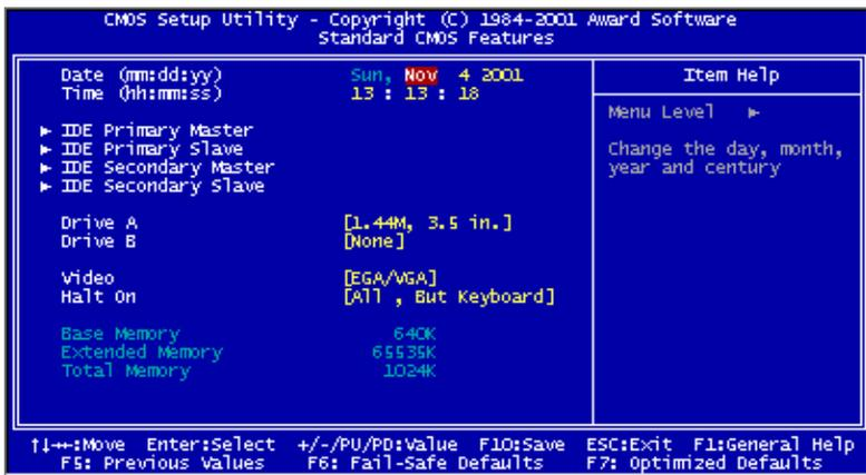
This standard setup menu allows users to configure system components such as the date, time, hard disk drive, floppy drive, display, and memory. Online help for each field can be accessed by pressing F1.
