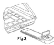
2. Fully insert your EC400 into the ExpressCard slot on your laptop and put the antenna in the up position as shown in Figure 3.
