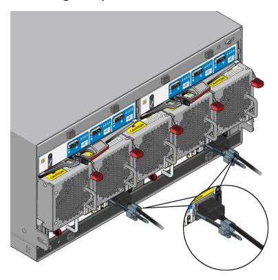
Figure 3. Securing the power cables
