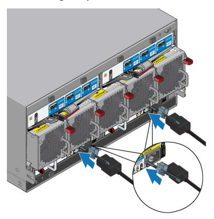
Figure 2. Connecting the power cables
