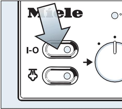
The **I-O** "On-Off" switch is used for switching the ironer on and off.
