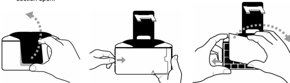
2. To Close: Slide the tab right to unlock the keyboard, snap keyboard shut, depress stand with thumb and secure.
