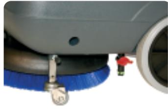
The built-in parking prop and wheel takes the weight off the brush and supports the machine when parked
