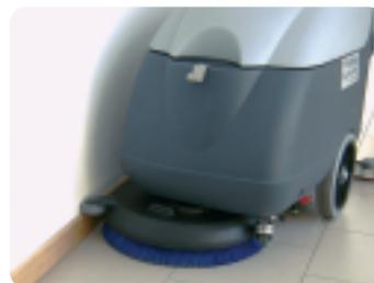
The offset brush deck with side wheel permits efficient close-up cleaning without damaging walls and furniture
