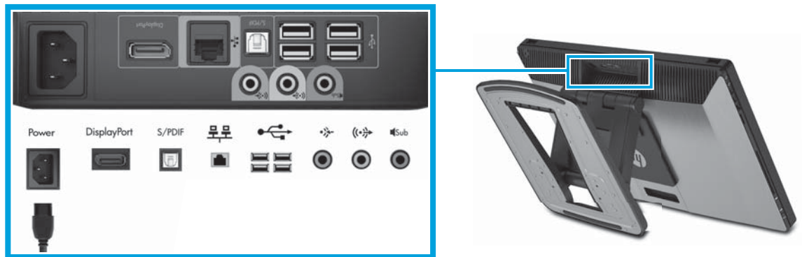
Figure 3-4 Connect cables to lower I/O panel
