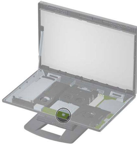
Figure 3-15 Internal USB port
