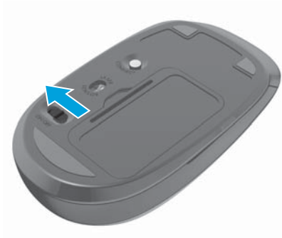
Figure 3-9 Turn switch on
