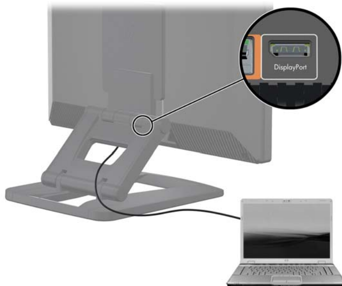
Figure 3-17 Connecting the display ports
