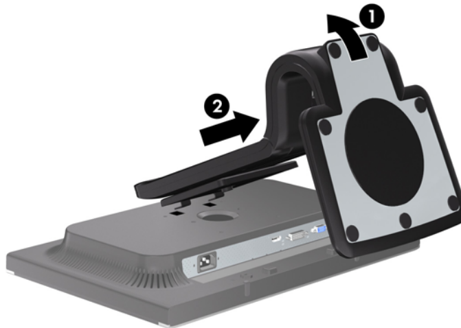
Figure 2-10 Removing the Pedestal Base
