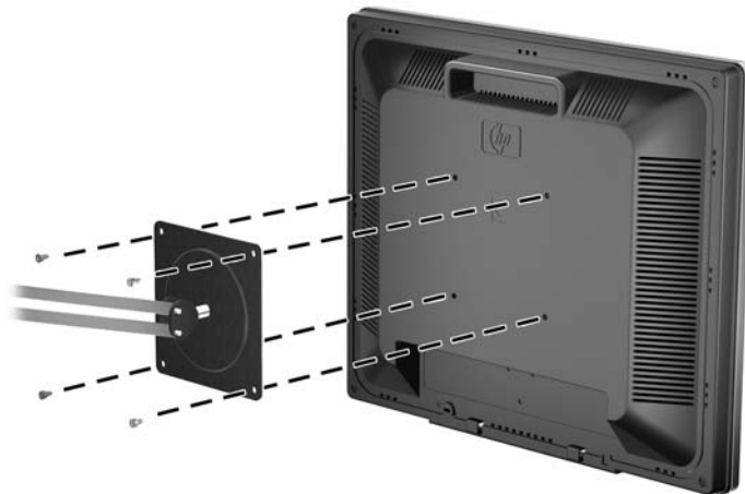
Figure 3-7 Installing the Monitor on a Swing Arm
