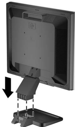
Figure 3-1 Attaching the Base to the Monitor
