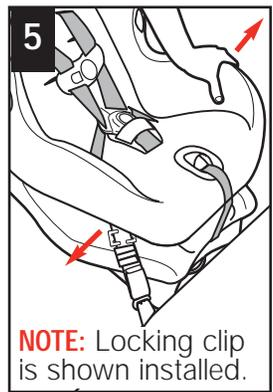
5 With weakest hand at belt path, tilt and push the child restraint forward and back, and from side to side. If the seat belts do not loosen, your child restraint should be secure.
