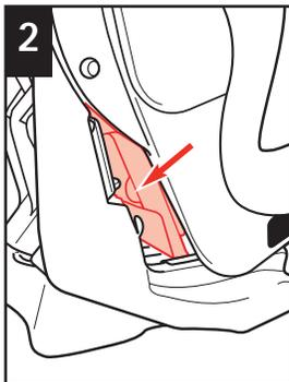
2 Place the child restraint into the reclined position. Locate the harness guard door and open it by pressing in on the door's tab.
