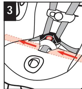
**3** Thread UNDER seat pad behind the crotch strap, between crotch strap and rear harness slot, and out opposite side. Buckle vehicle belt.
