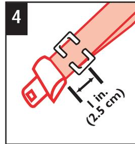
4 Position locking clip about 1 in. (2.5 cm) from vehicle belt's buckle plate.
