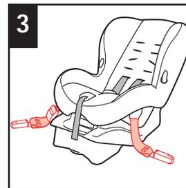
3 Adjuster **MUST** be on the **left side** of child restraint as shown. **DO NOT** twist belt.
