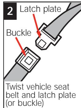
the buckle plate over. If the buckle slides, turn the buckle. Refasten the vehicle lap belt. The release button should face **out** after twisting so that it is easy to reach in an emergency.
