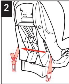
2 Adjuster **MUST** be on the **left side** of child restraint as shown. **DO NOT** twist belt.
