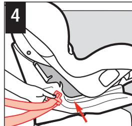
4 Thread the vehicle lap belt or lap/shoulder belt combination through the belt path and out other side. Buckle.
