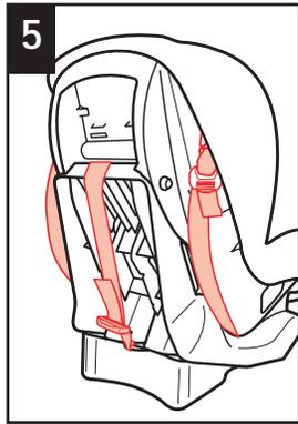
5 When LATCH is not being used, fasten LATCH hooks on side of child restraint as shown. Hook top anchorage strap to recline foot (see "Adjusting the Top Anchorage Strap" section).
