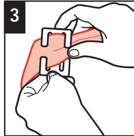
3 Thread both portions of the vehicle belt onto the locking clip.
