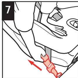
7 Push down firmly on the child restraint and pull up on the loop to tighten belt.
