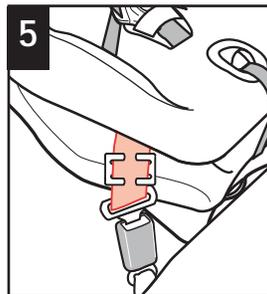
5 Rebuckle belt. Lap belt portion should now be tight. If not, remove locking clip and repeat all steps.
