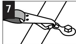
7 With knee still in child restraint, attach hook to anchor in vehicle. Push down firmly and tighten top anchorage strap. To adjust top anchorage strap: See "Adjusting Top Anchorage Strap" section.
