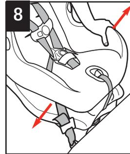
8 With weakest hand at belt path, tilt and push the child restraint forward and back, and from side to side. If the LATCH belts do not loosen, your child restraint should be secure.
