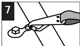
**7** With knee still in child restraint, attach hook to anchor in vehicle. Push down firmly and tighten top anchorage strap.
