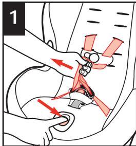
1 Loosen harness by pushing down on the harness release lever while pulling out on the harness. Undo harness retainer and unbuckle the buckle.
