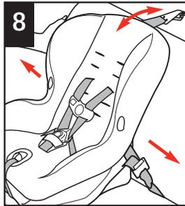
With weakest hand at belt path, tilt and push the child restraint forward and back, and from side to side. If the LATCH belts do not loosen, your child restraint should be secure.
