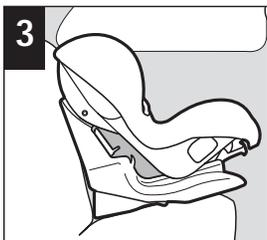
3 Place child restraint **flush** against the back of the vehicle seat **forward-facing** in the back seat.
