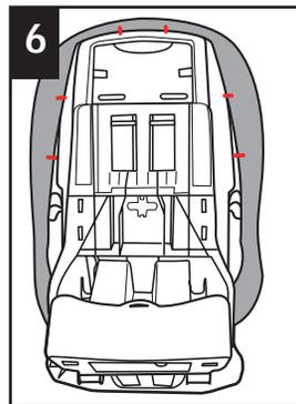
6 From the back of the restraint, pull pad out from the tabs (shown in red).
