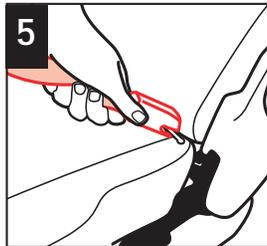
5 Fasten one LATCH belt connector to the anchor in the vehicle seat located in the vehicle seat bight. Repeat for other side of child restraint. See your vehicle owner's manual for more information.
