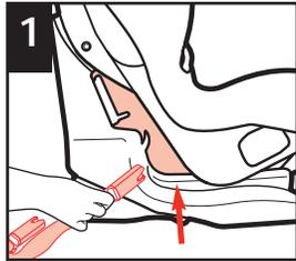
1 Recline child restraint. To thread the LATCH belt, put belt end with connector and adjuster through the forward-facing belt path slot.
