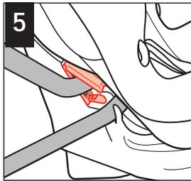
**5** Thread the shoulder belt through the lock-off on the **opposite side of the vehicle buckle**. Close the lock-off. Lock by lifting up the tab to the locked position.
