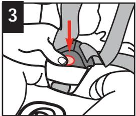
3 Press red button on buckle to release the buckle plates. Place harness over sides of child restraint. Remove child.
