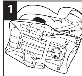
To move the recline foot to the rear-facing position, lay restraint on it's side.
