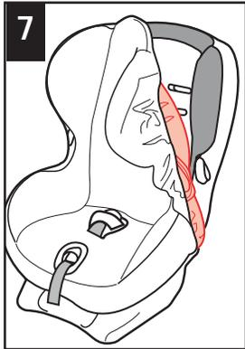
7 From the front, pull pad off the shell, starting at the top. Lift pad over the harness strap holders and work the pad around the harness adjustment cover.
