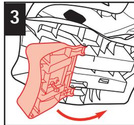
3 Rotate the recline foot to the back of the restraint and lock into place.
