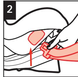
**2** Thread the vehicle lap or lap/shoulder belt combination through the rear-facing belt slot.
