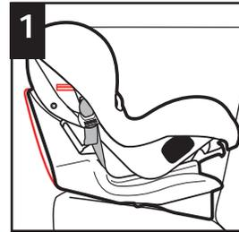
**1** Place child restraint rear-facing in the back seat. With child restraint in the fully reclined position, make sure level line on side of shell is level with ground. Adjust child restraint if needed.
