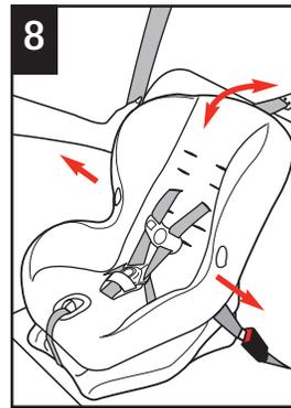
**8** With weakest hand at belt path, tilt and push the child restraint forward and back, and from side to side. If the seat belts do not loosen, your child restraint should be secure.
