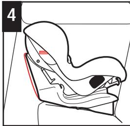
4 Place child restraint rear-facing in the back seat. With child restraint in the fully reclined position, make sure level line on side of shell is level with ground. Adjust
