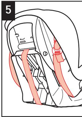
**5** When LATCH is not being used, fasten LATCH hooks on side of child restraint as shown.
