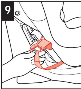
Pull out the harness and splitter plate.
