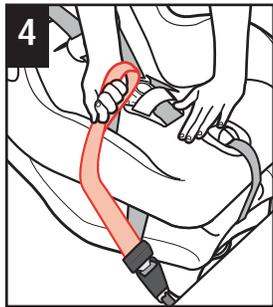
4 Push down firmly on the child restraint and pull up on belt to tighten. For a manual belt, refer to "Knowing your Vehicle Belt" section. Pull up on shoulder strap to remove any slack.
