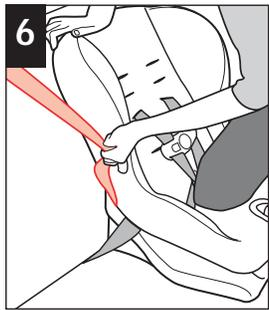
**6** Place one knee in the child restraint and push down firmly while pulling up on shoulder belt to tighten. For a manual belt, refer to "Knowing your Vehicle Belt" section.
