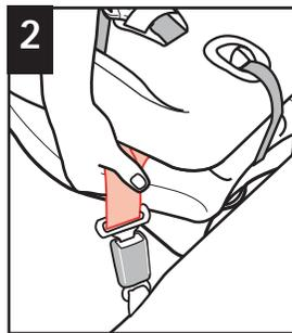
2 Grasp both vehicle belts together just behind the buckle plate and unbuckle. **NOTE:** If the buckle plate ends up behind the child restraint, grasp the belts to the outside of the child restraint, as close to the buckle plate as possible.
