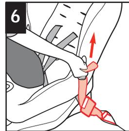
6 Place one knee in the child restraint and push down firmly while pulling up on loop end of the LATCH belt to tighten.
