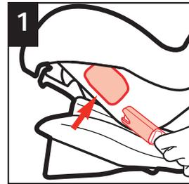
1 To thread the LATCH belt, put belt end with connector and adjuster through the rear-facing belt path slot.
