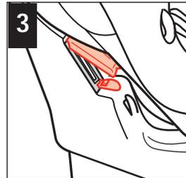
3 Open the lock-off opposite of the vehicle buckle by press down on the lock-off's tab.
