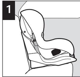
1 Place child restraint **flush** against the back of the vehicle seat **forward-facing** in the back seat.
