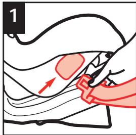
1 Thread both vehicle lap and shoulder belts through the slot (as shown) and out other side. Buckle. Pull up on shoulder belt until all slack is out and lap belt is tight.
