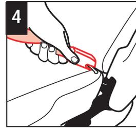
4 Fasten one LATCH belt connector to the anchor in the vehicle seat located in the vehicle seat bight. Repeat for other side of child restraint. See your vehicle owner's manual for more information.
