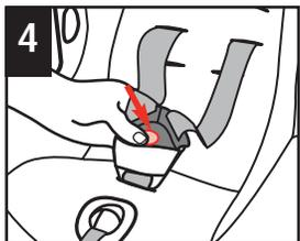
**4** Press red button on buckle to release the buckle plates. Hook harnesses on the harness strap holders on the sides of child restraint.
