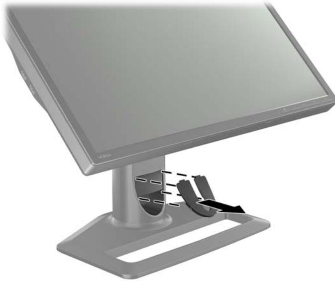
2. Before connecting the cables, route them through the cable routing hole in the column (1) and replace the cable routing cover (2).
