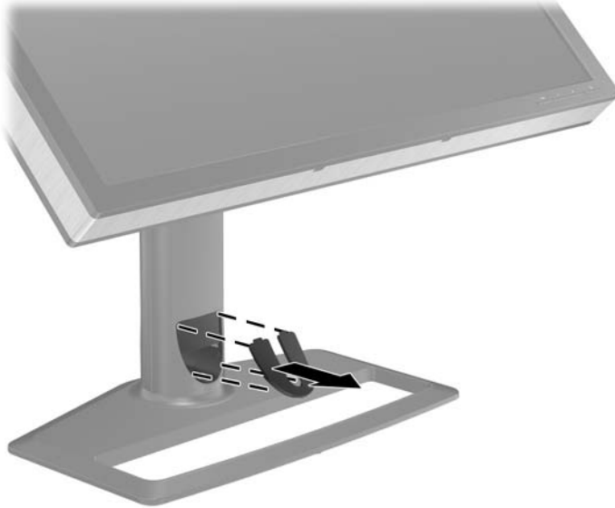
Figure 3-3 Removing the Cable Routing Cover
