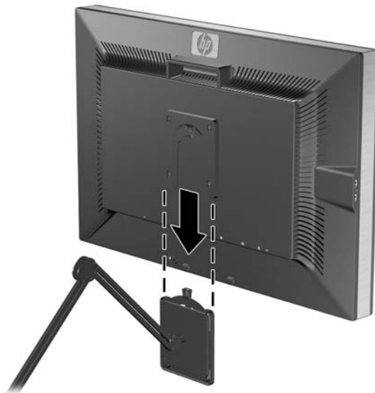
Figure 3-13 Inserting the Monitor Panel into the Quick Release
