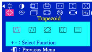
The **Trapezoid** parameter allows you to adjust the trapezoid settings when the top or bottom of the picture is too large or small.
