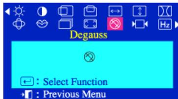
The **Degauss** parameter allows you to remove color impurities caused by magnetic fields. Do not use the **Degauss** feature more than once within a 30-minute period.
