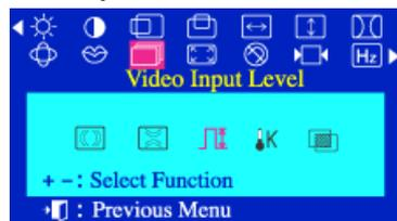
Some video cards use video signals higher than 0.7 V which causes the display to be very bright. The normal level used for most PC's is 0.7 V. The **Video Input Level** parameter allows you to select the level that is best suited to your computer's video card.
