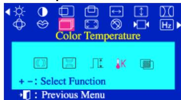
The **Color Temperature** is a measure of the "warmth" of the image colors. The available range is from -6500 to 9300K.
