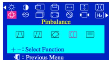
The **Pinbalance** parameter allows you to adjust the pinbalance setting when the sides of the picture are bowed towards the left or right.
