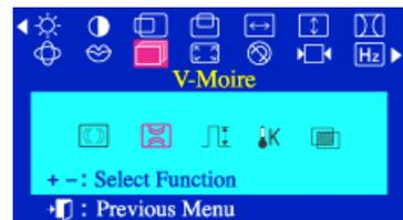
The **Vertical Moire (V-Moire)** parameter allows you to correct your picture's vertical moire pattern.
