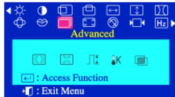
The **Advanced** parameter allows you to access the following parameters: **H-Moire**, **V-Moire**, **Video Input Level**, **Color Temperature** and **Halftone**.
