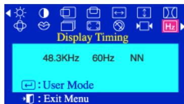
The **Display Timing** parameter allows you to display your monitor's settings.
