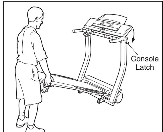
2. Move your right hand to the position shown and hold the treadmill firmly. Using your left hand, pull the storage latch to the left and hold it. Raise the treadmill until the catch plate is past the pin on the storage latch. Slowly release the storage latch. **Make sure that the pin is securely holding the catch plate as shown.**
