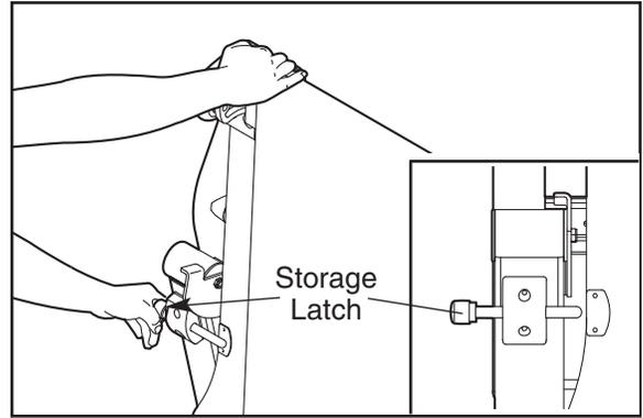
2. Hold the treadmill firmly with both hands, and lower the treadmill to the floor. **CAUTION: To decrease the possibility of injury, bend your legs and keep your back straight. Do not drop the treadmill.**
