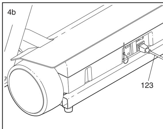
5. Locate the indicated wire on the back of the cabinet. Plug the wire into the connection panel.
