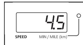
To stop the walking belt, press the Stop button. The Time/Segment Time display will begin to flash. To restart the walking belt, press the Start button or the Speed + button.
