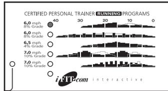
The console features four jogging programs and five running programs. The profiles on the console show how the speed and incline of the treadmill will change during the programs. The numbers beside the profiles show the maximum speed and incline settings for the programs.
