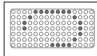
**Distance/Incline/Laps display—**This display shows the distance that you have walked, the incline level of the treadmill, and the number of
