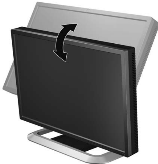
Figure 3-7 Tilting the Monitor
