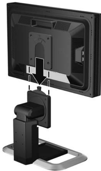
Figure 3-1 Inserting the Monitor into the Pedestal Base
