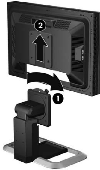
Figure 3-12 Removing the Monitor from the Pedestal Base
