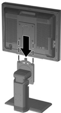
Figure 3-1 Inserting the Monitor into the Pedestal Base
