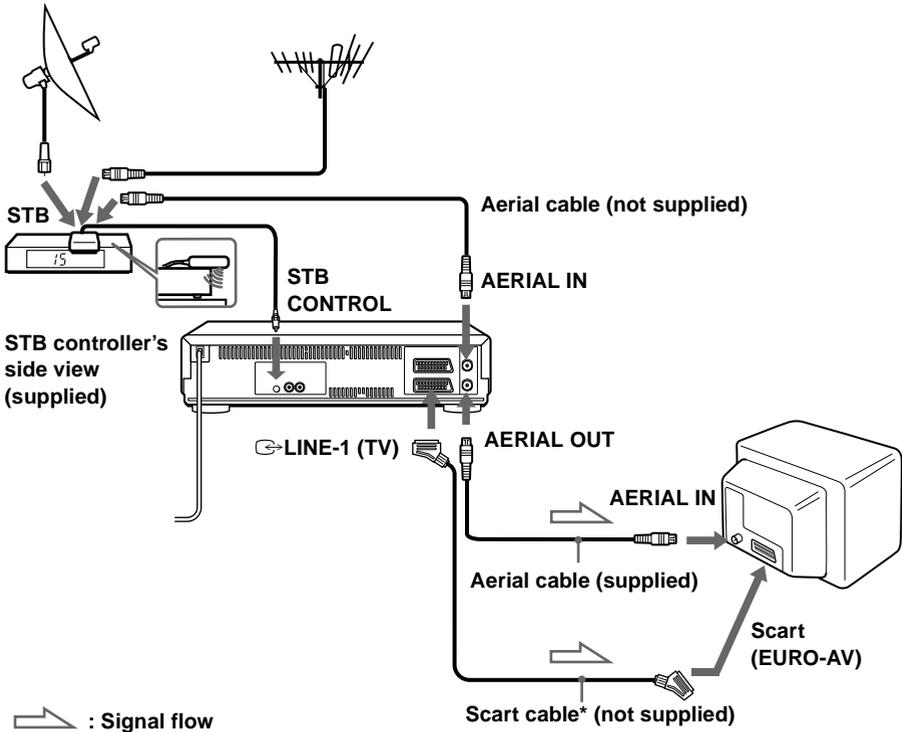
\* If your TV does not have a Scart (EURO-AV) connector, the Scart cable connected to the VCR is not required.
