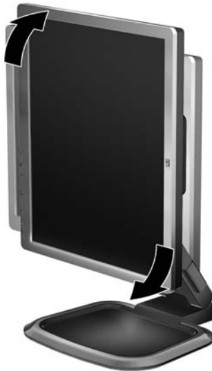
Figure 3-10 Pivoting the Monitor
