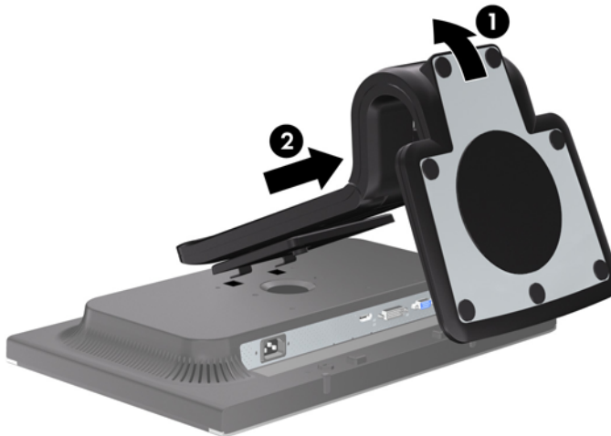
Figure 2-10 Removing the Pedestal Base
