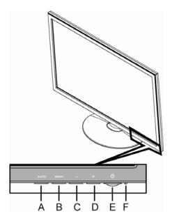
Auto button Α Automatically fine-tunes the image quality. В Menu button Opens, selects, or exits the OSD menu. C - (minus) button Navigates backward through the OSD menu and decreases adjustment levels. D + (plus) button Navigates forward through the OSD menu and increases adjustment levels. Ε Power button Turns the monitor on or off. F Power LED Fully powered = green Sleep mode = amber
