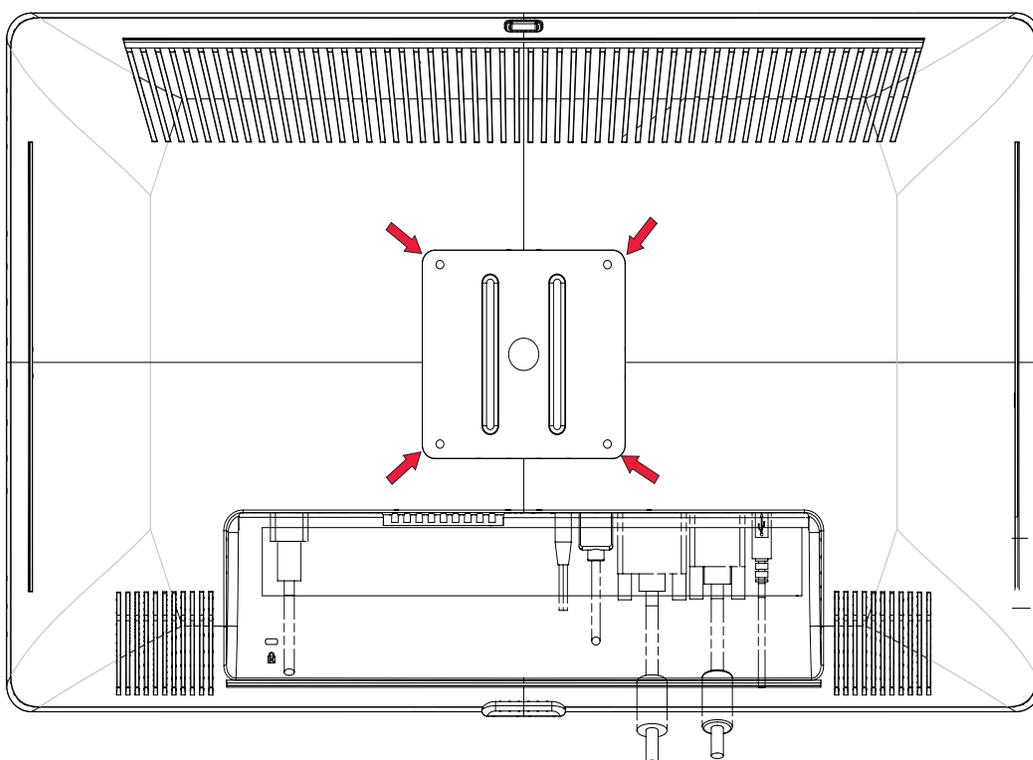
*Threaded holes for attaching wall mount*
