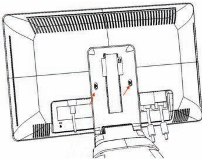
*Removing the plate from the back of the monitor*
