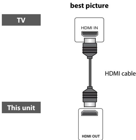
When connecting with an HDMI cable, the audio signal will be output as the digital audio signal simultaneously, so you do not need the analog audio connection described on page 6.
