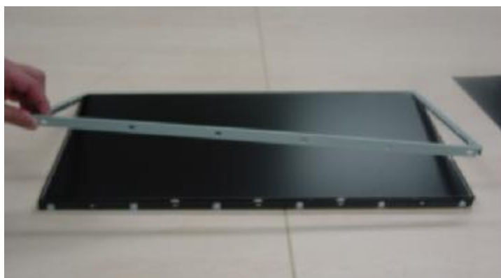
Step7 : Separate case top(push the case top because of damages on COF)
