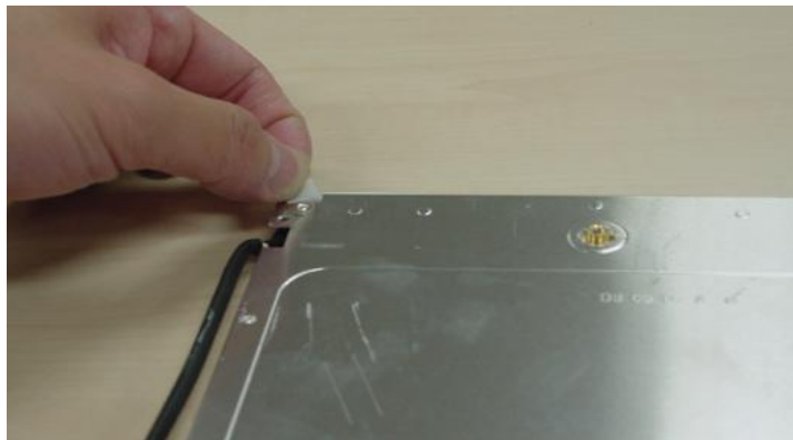
Step13 : remove lamp wire tapes (left/right)
