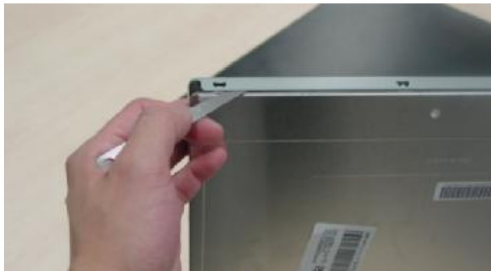
Step5 : Dismantle the case top(Down)
