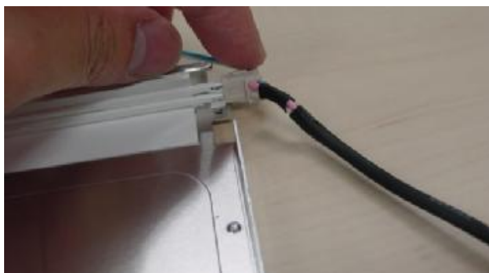
Step15 : Separate Lamp holder(H) from holder Guide of Cover bottom
