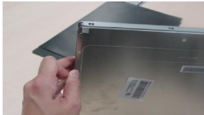
Step6 : Dismantle the case top(left/right)
