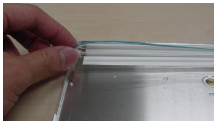
Step16 : Separate Lamp holde(G) from holder Guide of Cover bottom.
