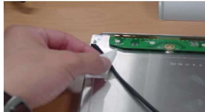
Step 4 : Separate wires from the tape
