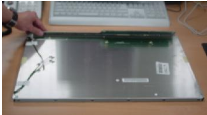
Step 3 : Remove the Cover Shield
