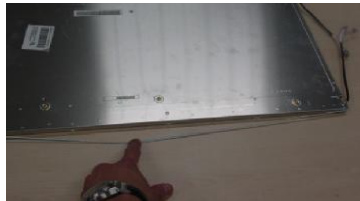
Step14 : Separate wires from Cover bottom
