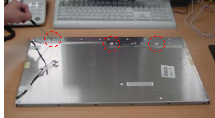
Step 2 : Unfix the screws (3 Points)
