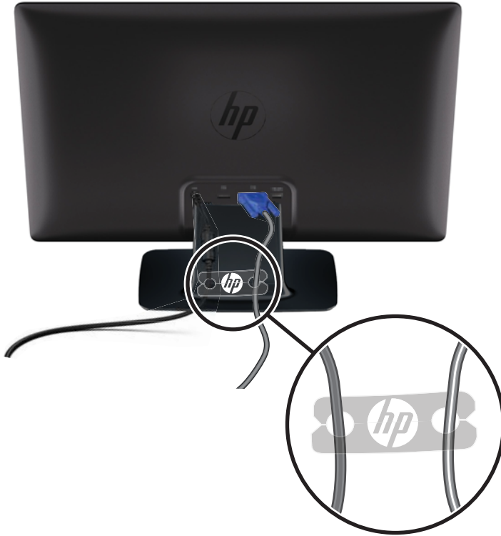
Figure 3-7 Installing the Cable management Clip
