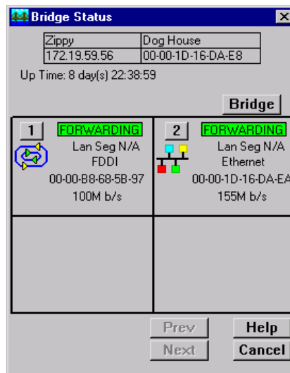
Figure 5-1. The Bridge Status Window
