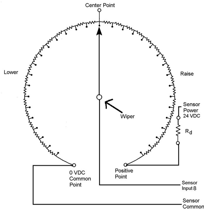
Figure 3-8: Typical OEM Potentiometer Powered by LTC-MAP
