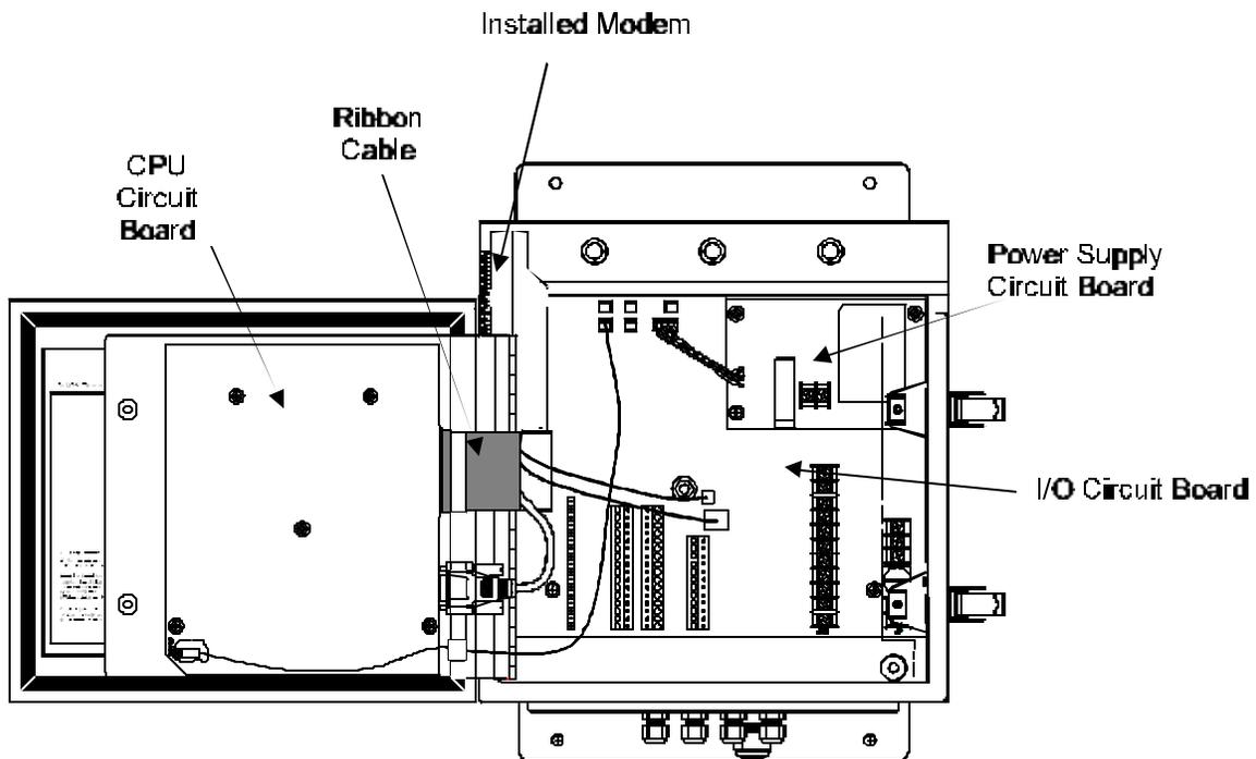
Figure 2-4: LTC-MAP 2130 (Top View with Face Panel Open)
