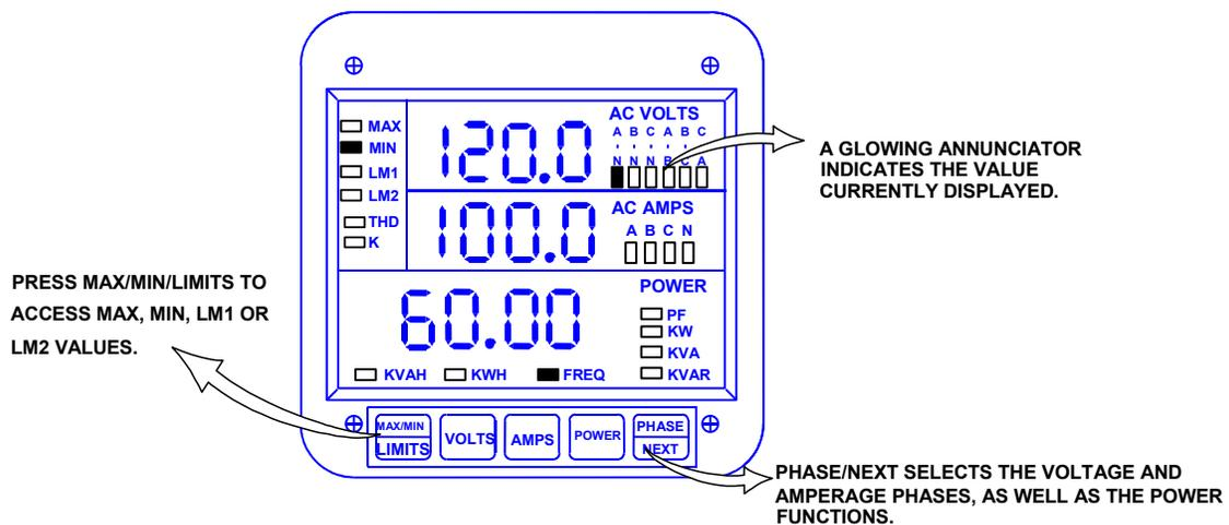
**Figure 5.1:** The EPM 5300P front panel with display and keypad
