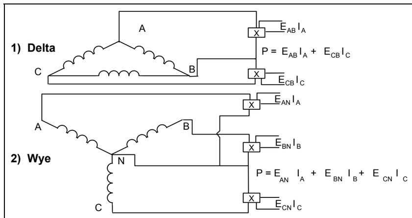
Figure 1.4: Poly Phase System: (1) Delta, (2) Wye
