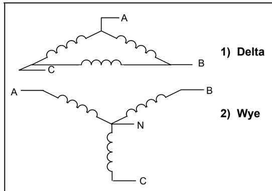
**Figure 1.3:** Three-Phase System: (1) Delta, (2) Wye
