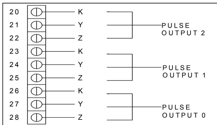
**Figure 3.2:** KYZ Relay Connection for -NL2 Option
