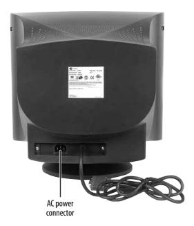
5 Plug the other end of the power cable into a correctly grounded electrical outlet.
