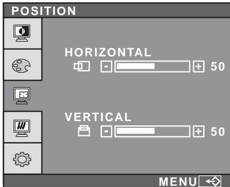
**HORIZONTAL.** Moves the display image left and right.
