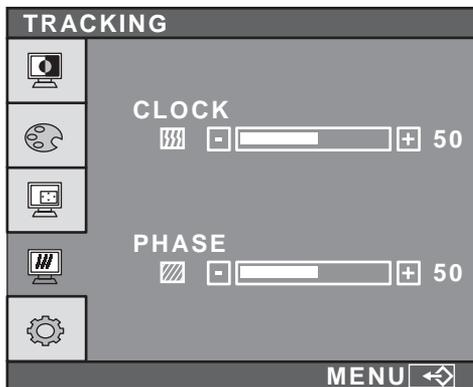
**CLOCK.** Minimizes any vertical bars or stripes visible on the screen background. The horizontal screen size will also change.
